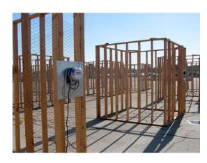
SCE constructed 40 structures at a facility located in Alhambra CA. These structures are wrapped in chicken wire and were designed to simulate residential home construction to provide a unique and flexible test site.
