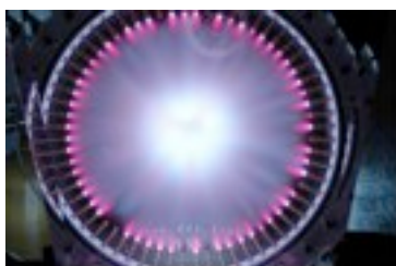
Figure 2. Convergence of plasma jets to form an imploding plasma liner. (Witherspoon et al. [25])
