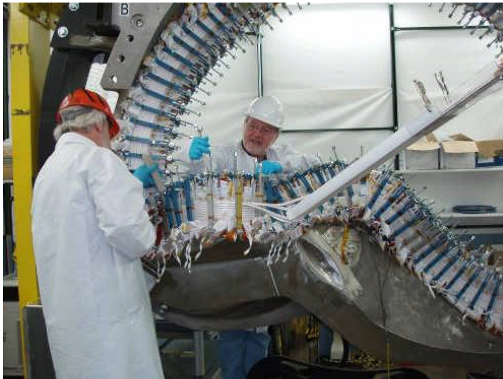
Figure 15: Modular coil winding operations at PPPL.
