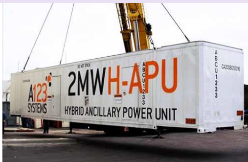
Ai23 Energy Storage System Container
